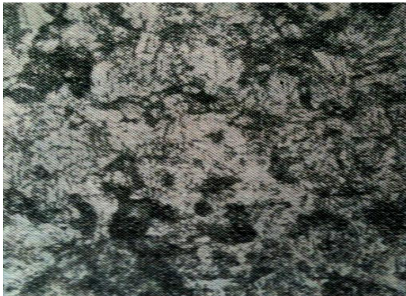
Fig.3 500×4% alcohol, nitric acid corrosion materials organizations: ferrite + graphite
