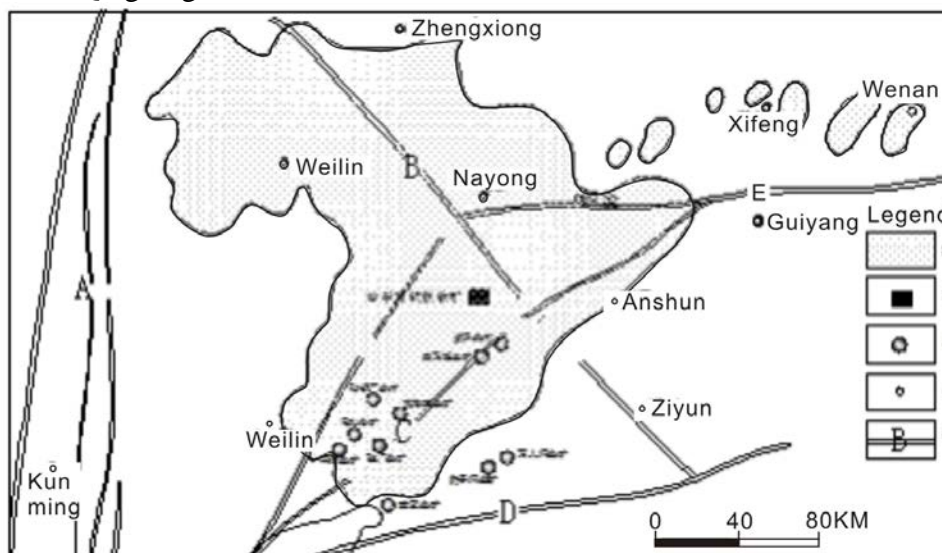
Fig.1 Geology map of the study area (based on, [1-2],[5-6],[10] revision);1 Large distribution of Emeishan basalt in Guizhou province; 2 scandium anatase ore; 3 laterite gold deposit (point); 4 Geographical names of the cities and counties; 5.Deep fracture zone and fracture zone A Xiaojiang fault B Shuicheng-Ziyun fault C Mile-Shizong fault D Nanpan River fault E Nayong-Anshun fault (based on Luo Yaonan, 1985, Gao zhenmin, Li Hongyang, 2002, Regional geology of Guizhou province 1987, Wang Yangeng, Chen Ivan, 2000 revision)
