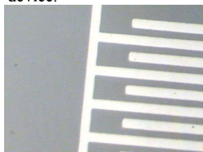
Figure 2. the top view IDTs photographic of the fabricated SAW device.
