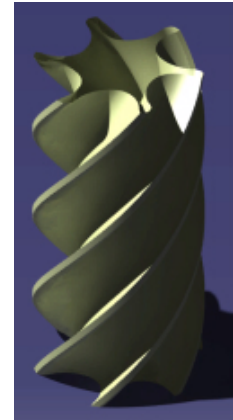
Figure 6. 3D modeling of screw compressor rotor
