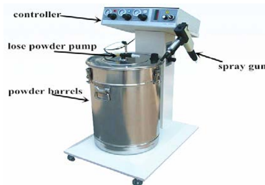
Fig. 4 Electrostatic spraying experimental apparatus
