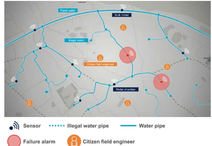
Figure 1: Illustration of the Citizen Field Engineer concept applied on a generic map over a water distribution network in a slum area. The illustration is a derivative of the OpenStreetMap. Copyright: OpenStreetMap contributors.
