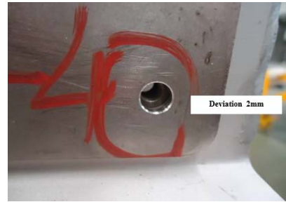
Figure 8. 4th hole of 3rd Cabinet has 2mm deviation
