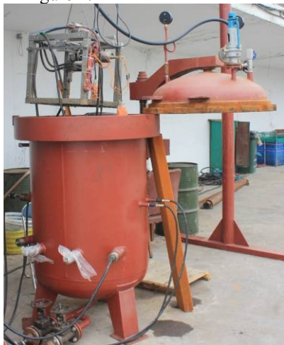
Figure 1. The pressure chamber and automatic welding equipment
