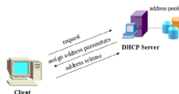
Fig. 1. Structure of DHCP system
