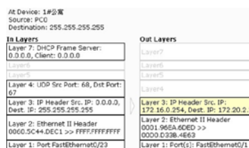
Fig. 5. Discover with relay address
