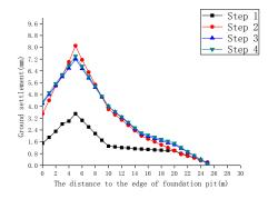
Figure 6. The curve of ground settlement.
