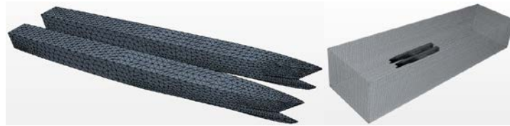
Fig. 3 The surface mesh and computed domain of model without SSB
