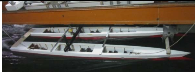
Fig. 1 Model test of ordinary catamaran
