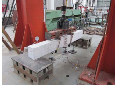
Figure. 2 Load device diagram of specimens
