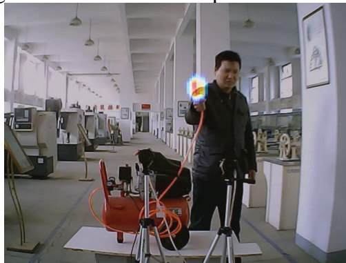
Fig.11 gas-leakage location by acoustic imaging
