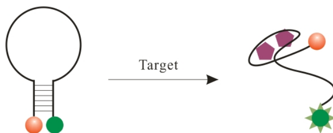
Fig. 1. Scheme illustration of operation principle of the developed aptasensor.
