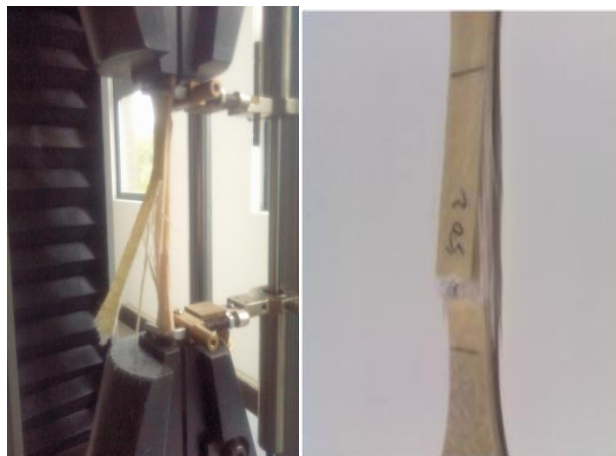
Fig.5 Tensile Failure of Samples
