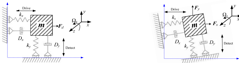
a. Idealized equivalent dynamic model
