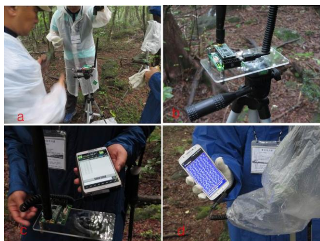
Figure4. Testbed: Halla mountain in Jeju Island (a) raining day, 925MHz band, over 200M (b) Sending node (c)(d) receiving node: check RSSI of receiving packets
