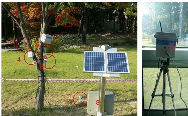
Figure 3. Testbed: Daejeon ETRI 1.Soil moisture 2.leaf wetness 3.diameter 4.temperature-humidity 5.Illumination/insolation 6.Co2 7.Sensor node 8.Battery module 9.Gateway: in-door
