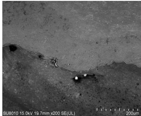
Fig.1 Microstructure with wavy interface after explosive welding
