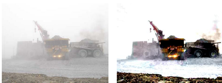
Fig. 1. The image recovery and enhancement under dust condition for haul trucks
