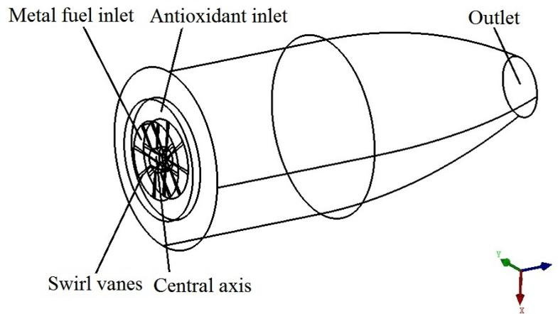
Fig. 2 Combustor structure
