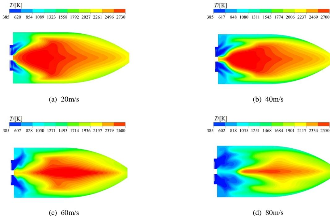
Fig. 5 The temperature field of four cases in YOZ surface
