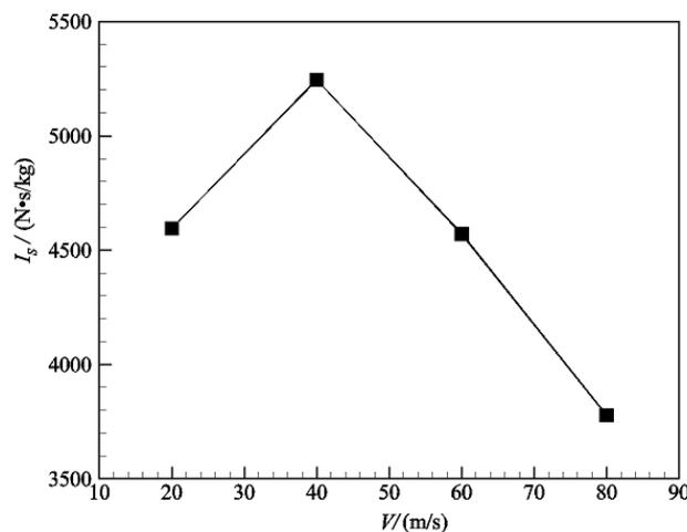
Fig. 8 The specific impulse at different inlet velocities
