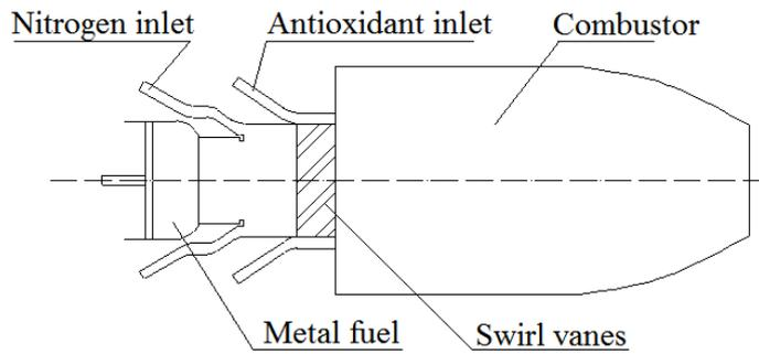
Fig. 1 A sketch of fuel supply system and combustor
