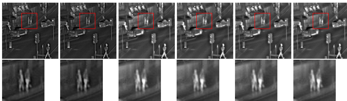
Fig. 4. The fused images of an infrared and visible image pair: the i -th column is obtained by using the combination of low and high frequency rules shown in the i -th row of Table 1.
