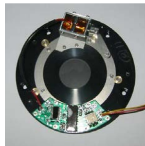
Figure 2. Mechanical shutter to control dosing time
