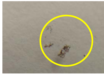
Figure 9. Damaged Coating layer
