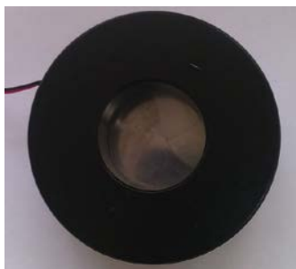
Figure 2. Mechanical shutter to control dosing time
