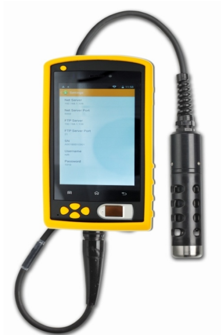
Figure 2 the portable rivers and lakes’ water quality on-line monitoring instrument physical map. the design of the portable rivers and lakes’ water quality on-line monitoring instrument
