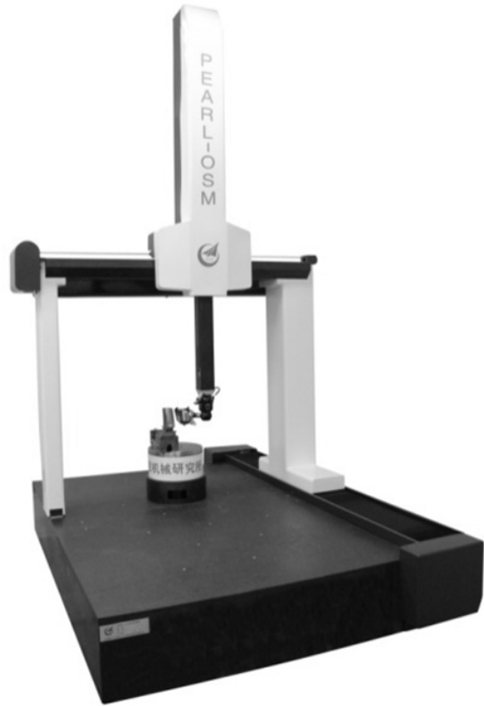
Fig. 1(b) Non-contact coordinate measurement system
