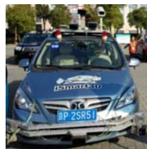
Fig.6.Ismart30 top eight LIDAR installation schematic diagram
