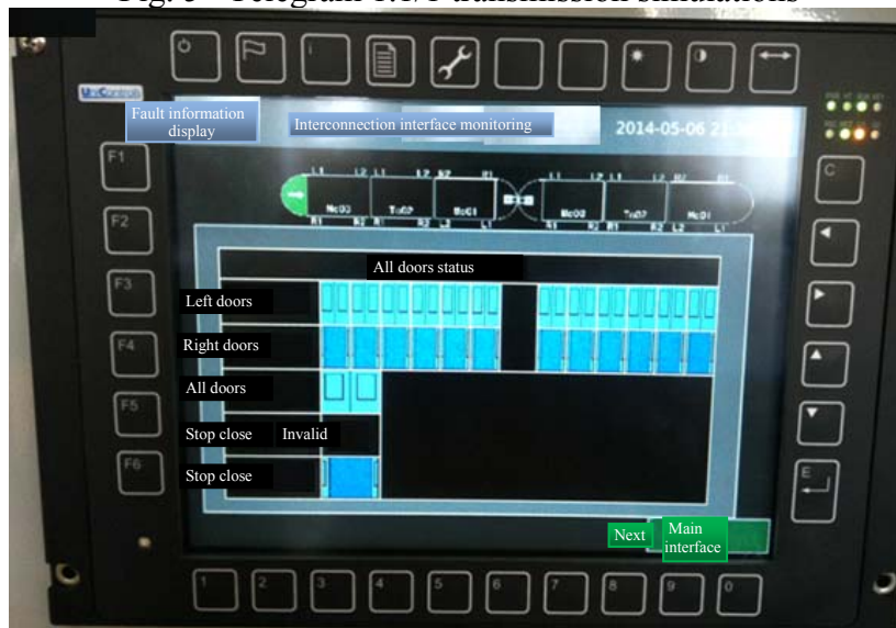
Fig. 6 Doors status display interface on HMI
