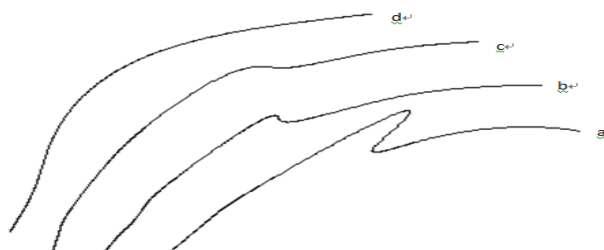
Figure 4 The comparison of cubic NURBS interpolation curve with weight factor given different values
