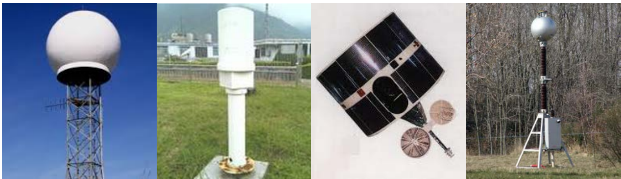
Fig.1. Common instruments to detect lightning. From left to right is the Doppler radar, lightning locator, meteorological satellite and atmosphere electronic field instrument.
