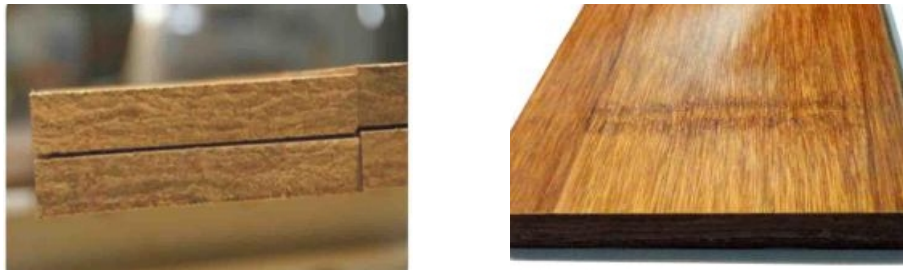
Fig.1 Section of bamboo steel material (left) and bamboo steel board (right)
