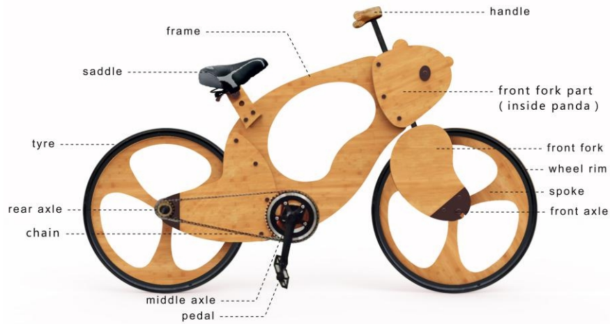
Fig.7 Appearance and name of each part of panda bamboo steel bicycle
