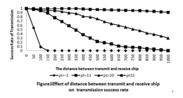
Figure 1 represents that the success rate of message transmission reliability reduces when the distance d increases, especially when the transmit power =3 dBm, link reliability decreased sharply with the increase of d.
