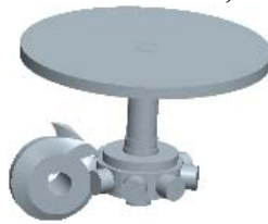
Fig.3, the 3D modeling of globoid cam indexing mechanism
