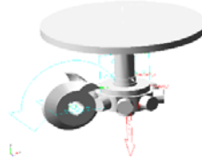
Fig.4, the multi rigid body virtual prototype of globoid cam indexing mechanism
