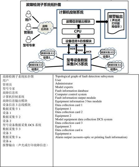
FIG 2 Composition block diagram of fault detection subsystem
