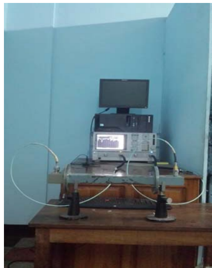
FIGURE VII. EXPERIMENTAL SETUP FOR WAVEGUIDE MEASUREMENT
