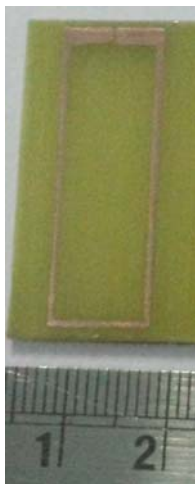
FIGURE VI. PHOTOGRAPH OF THE FABRICATED OLR
