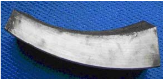
FIGURE VI. SAMPLE WITH THE TOP LEAD ARCHIMEDES SPIRAL AND THE BOTTOM LEAD CIRCLE CURVES
