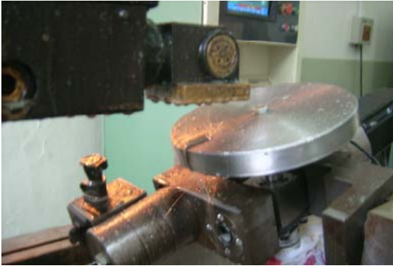
FIGURE V. MACHINING PROCESS OF THE SPATIAL CURVED SURFACE PARTS
