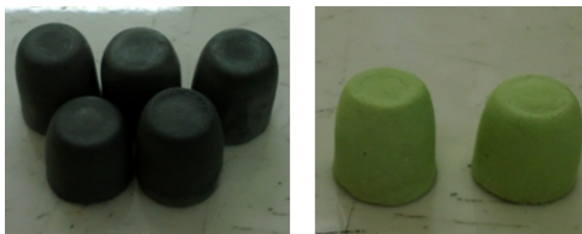
Fig.2 Green supports and supports after sintered at 1200°C
