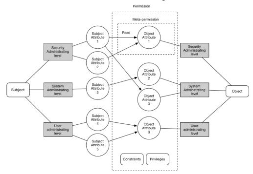
Fig.1 The framework of the TCBEAC model
