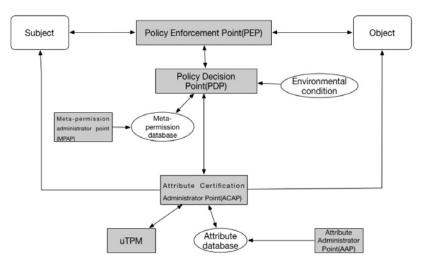
Fig.4 The framework of the TCBEAC system
