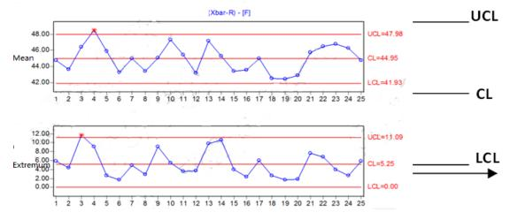
Figure 3. The mean range charts of sauce packet heat seal strength
