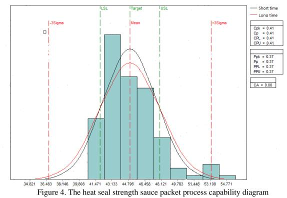
By the actual process capability figure shows, when the distribution center and the tolerance center does not coincide, in accordance with Cpk criterion for judging the value of the figure Cpk of
