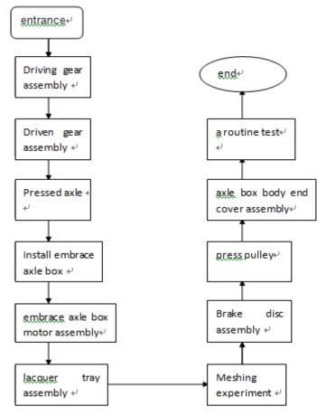
Fig. 1 HXD3B type drive unit assembly flow chart
