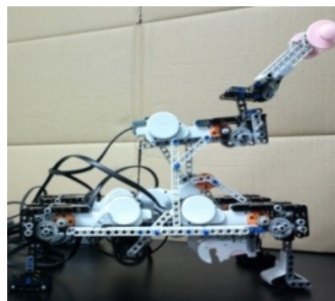
Fig. 2 The structure of the self-reconfigurable quadruped robot
