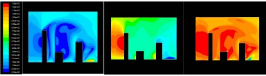
Fig.7 The distribution map of wind speed, pressure, temperature
