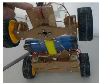
Fig. 3 Steering structure of experimental vehicle
