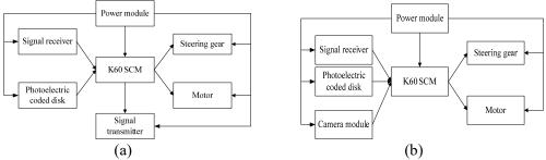
Fig. 1 Hardware control system structure of the front car and rear car
