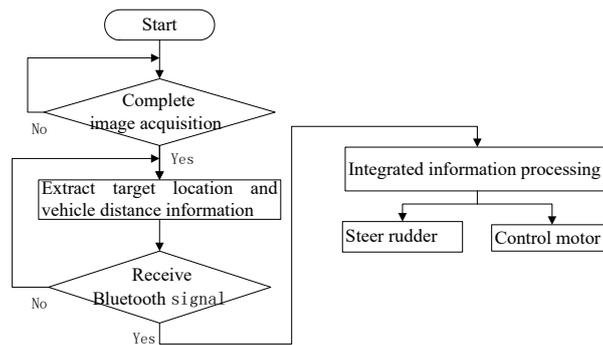
Fig. 4 Main program flow chart of rear vehicle
