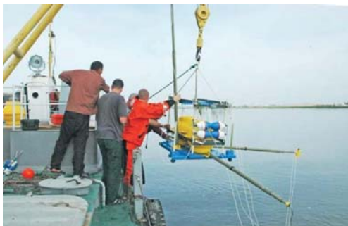
Fig. 5 Nord West Ltd. (Moscow, Russia) personnel deploy a shallow-water Marine MT system in the Caspian Sea.
