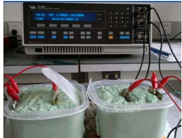
Fig.2 The complex impedance measurement system including the Solartron-1260A (on the desk), and wet flour dough mixed with copper sulfate to contact the non-polarizing electrode pair.
