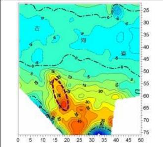
Fig.5. The trend analyzed magnetic anomaly contour map of the survey area in Lizhuang village, Hongchuan town(the oval line shows the location of the wreck).
