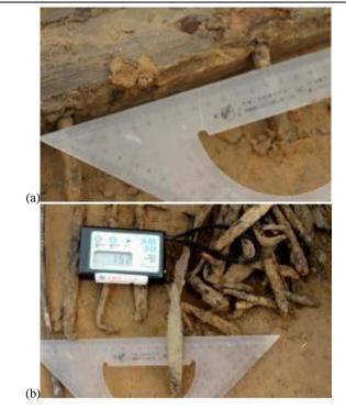
Fig.3. Phoenix Xiang ancient shipwreck on the iron claw nail distribution(a), specifications and magnetic strength test image (b) .The values in the table represent the intensity of magnetization rate , unit: 10-3SI.
