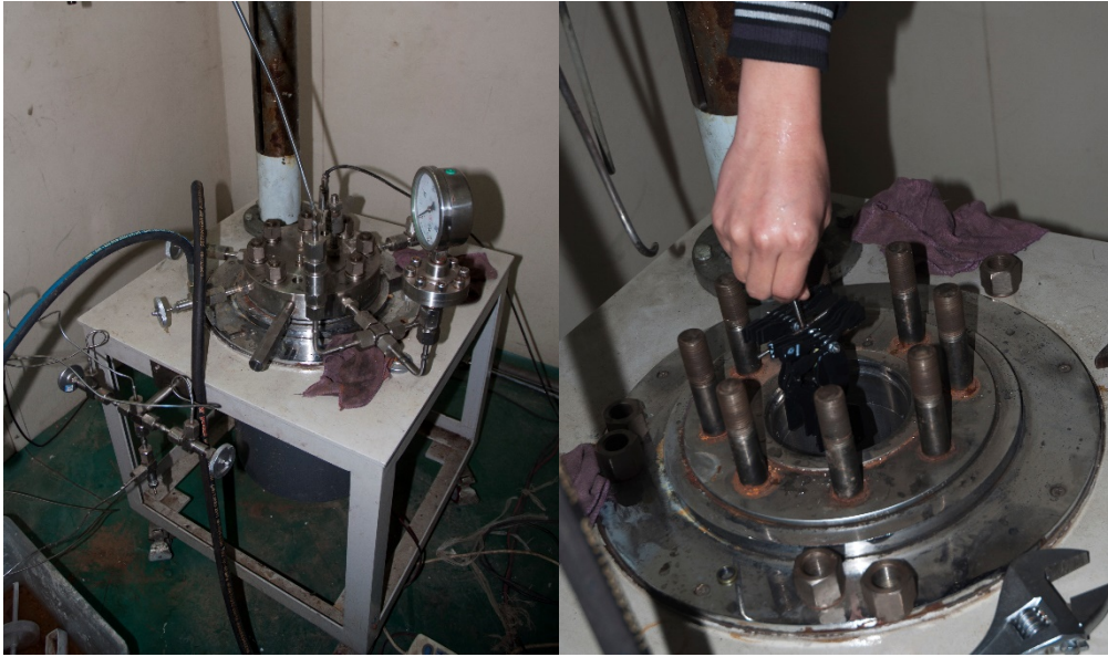
Fig. 1 High pressure autoclave for rubber resistance liquid test
