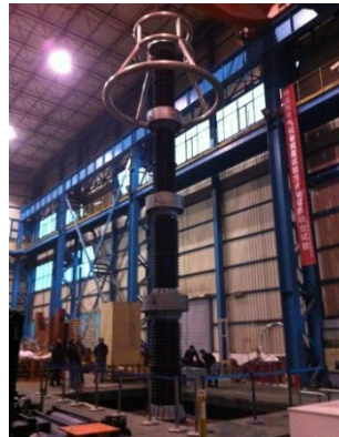
Figure 4. The shaking table test of 1000kV arrester
