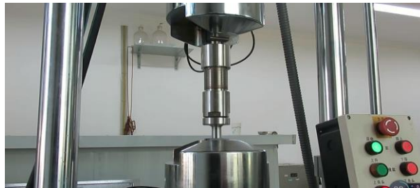
Figure 1. The mechanical test of mental damper
