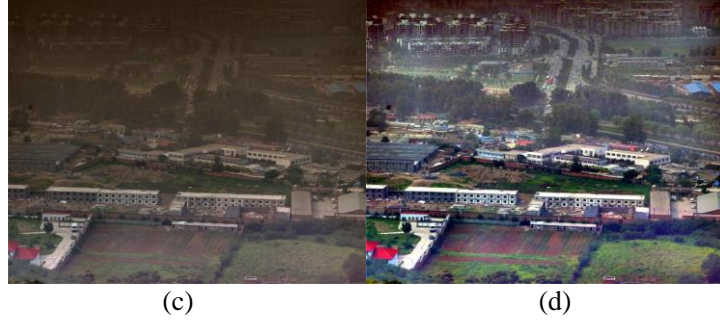
Fig. 4 experimental results;(a) Original image;(b) processed by SSR algorithm;(c)intermediate result by our improved algorithm;(d)final result by our improved algorithm.
