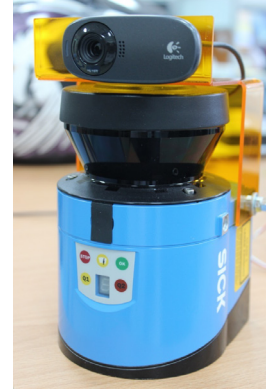
Fig. 1. An integrated multisensor system consists of a 2D laser scanner and a commercial webcam.
