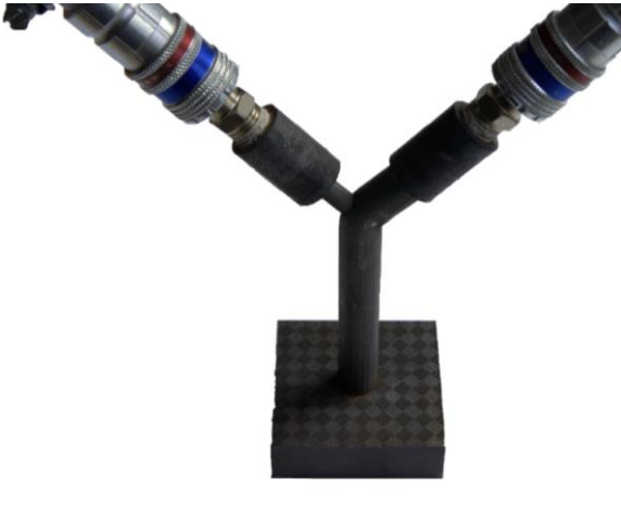
Fig. 5. The physical test objects for point cooling.
