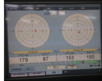
Fig. 10 Dynamic balancing correction results
