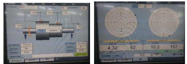
Fig. 9 Balancing parameter setting and measurement
