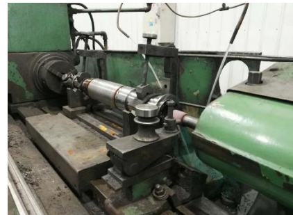
Fig. 6 Shaft assembly grinding
